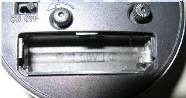
*The battery compartment and terminals after cleaning*
