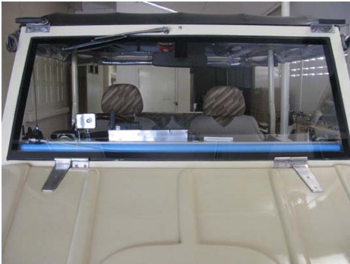
View from exterior front showing the blue PVC pipe cable tray and the tops of instruments on the over the dash mounting bar.
