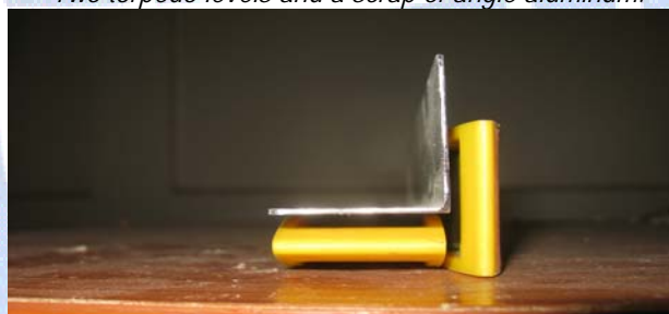
Glue the torpedo levels to the angle aluminum.
