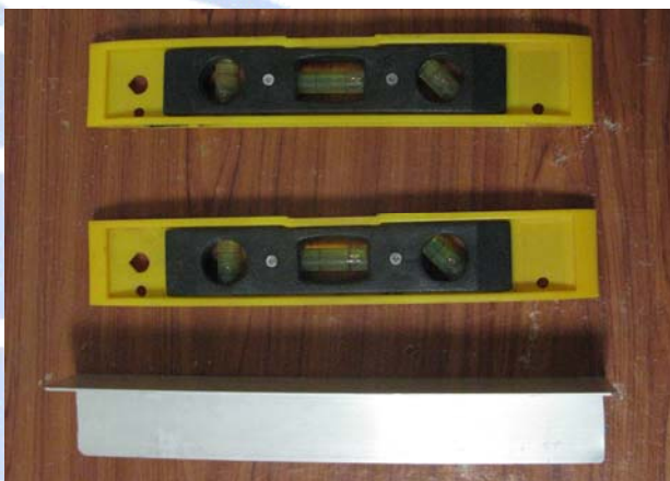
Two torpedo levels and a scrap of angle aluminum.
