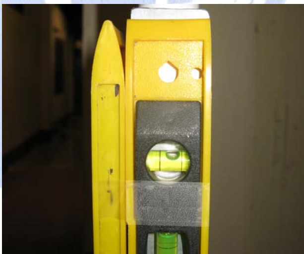
Watch the bubbles in the levels and adjust as needed.
